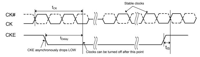
Figure 47. Clock frequency change in precharge power down mode
