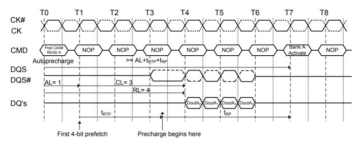
Figure 32.3. Burst read operation with auto precharge followed by activation to the same bank (t<sub>RC</sub> Limit): RL=5(AL=2, CL=3, internal t<sub>RCD</sub>=3, BL=4, t<sub>RTP</sub> 2 clocks)
