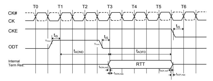
Figure 13. ODT timing for active standby mode
