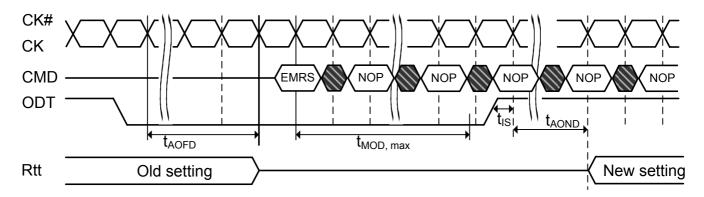
NOTE 1: EMRS command directed to EMR(1), which updates the information in EMR(1)[A6,A2], i.e. Rtt (Nominal). NOTE 2: "setting" in this diagram is measured from outside.
