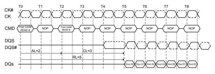
NOTE : The seamless burst read operation is supported by enabling a read command at every other clock for BL = 4 operation, and every 4 clock for BL =8 operation. This operation is allowed regardless of same or different banks as long as the banks are activated.
