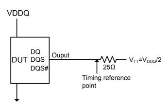
The output timing reference voltage level for single ended signals is the crosspoint with VTT. The output timing reference voltage level for differential signals is the crosspoint of the true (e.g. DQS) and the complement (e.g. DQS#) signal.
