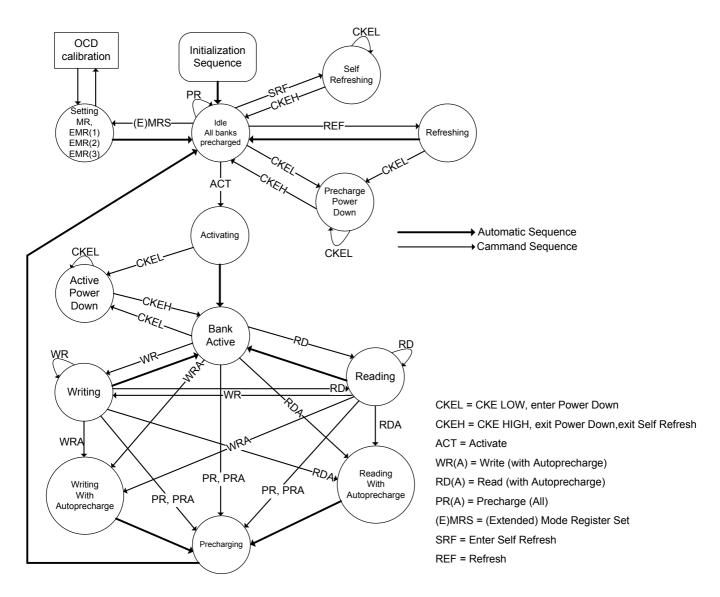
Note: Use caution with this diagram. It is indented to provide a floorplan of the possible state transitions and the commands to control them, not all details. In particular situations involving more than one bank, enabling/disabling on-die termination, Power Down entry/exit, timing restrictions during state transitions, among other things, are not captured in full detail.
