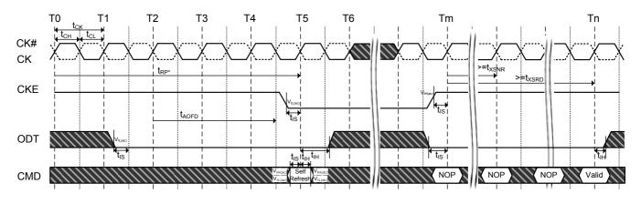
NOTE 1 Device must be in the "All banks idle" state prior to entering Self Refresh mode. NOTE 2 ODT must be turned off  $t_{AOFD}$  before entering Self Refresh mode, and can be turned on again when  $t_{XSRD}$  timing is satisfied.
